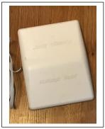
Small bed shaker "super shaker" by Sonic Alert (to be used with a Sonic Alert alarm clock) =>
